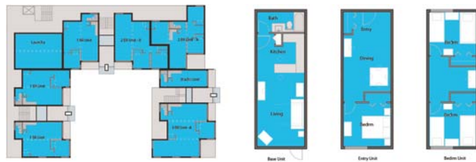
3. Spatial arrangements using three simple modular types to create a diverse mixed floor plan
