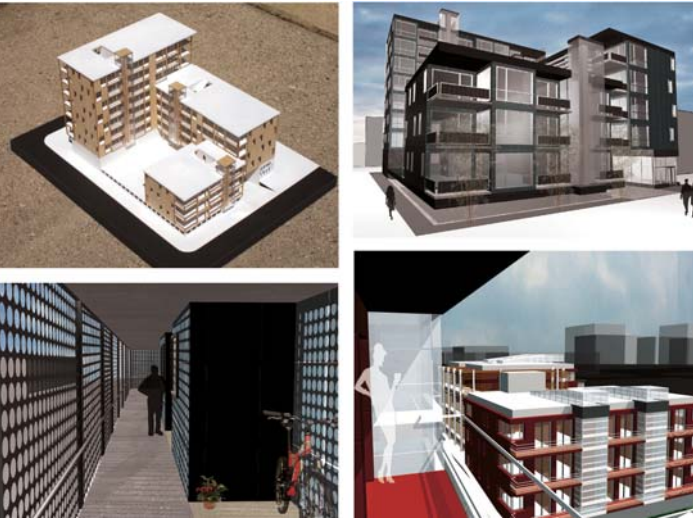
2. High-density housing concept examples in Detroit showing individual balconies and integral solar thermal flues including access corridors with semi private entrance areas, partially enclosed with translucent screens, providing a second “defensible space” communal balcony
