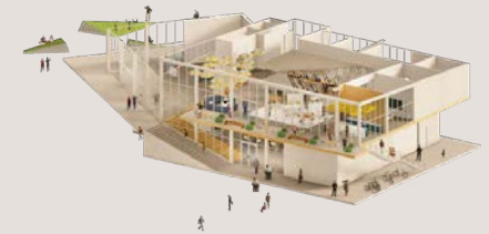
Split level plan navigates grade change and permits multiple access points for different user groups
