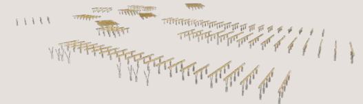
System of ground trusses and minimal concrete piers, reduces disruption to underground lava tubes
