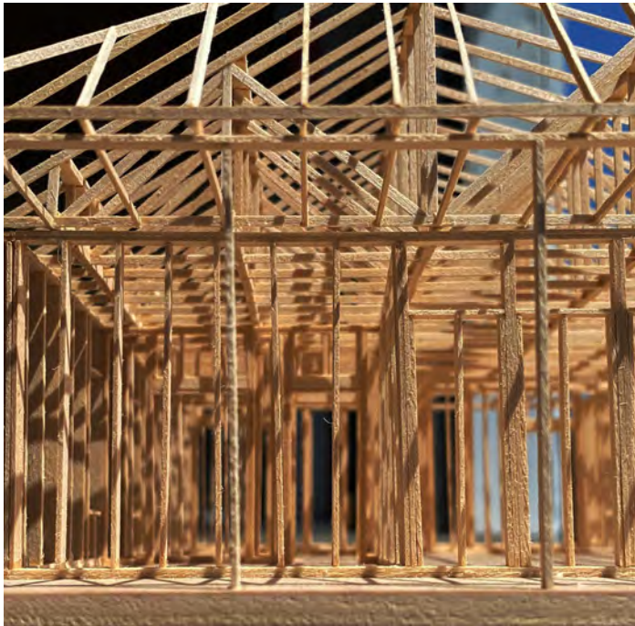
ABOVE: studies of construction material technologies and their impact on time and cost were studied during the design process of Timberlands Prototype 01; BELOW: framing model of the traditional stick-built construction strategy chosen for the initial prototype
