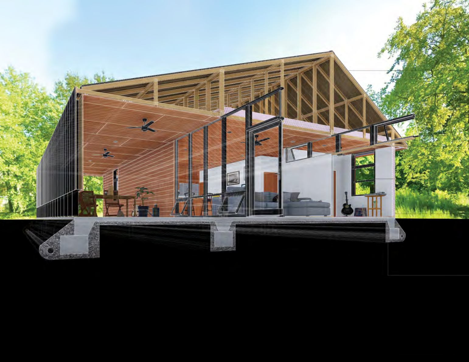
Section perspective drawing showing the interior of Timberlands Prototype 01, emphasizing the livability of the spaces as well as the benefit of cross ventilation through operable windows in the carport and bedroom.
