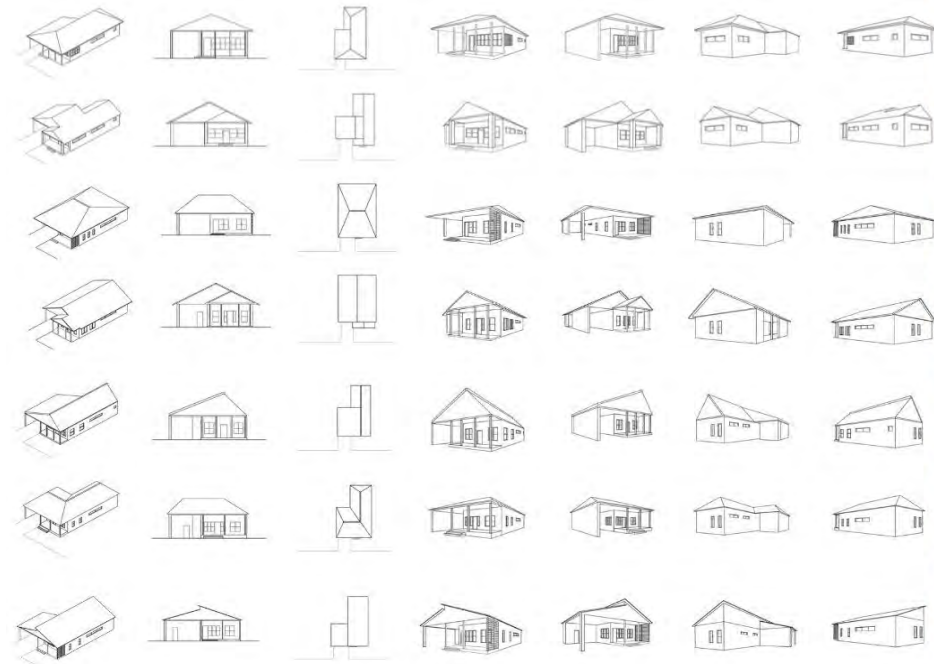
Iterative sketches and drawings of spatial organization, form, siting, massing, façade and fenestration informed by analysis and potential resident feedback.
