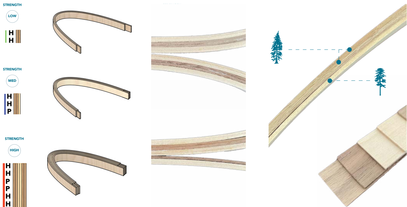
Figure 1. Strengths of laminates based on wood species (left), and physical studies (right). “H” denotes a layer of hemlock, “P” denotes a layer of pine. Jonathan Monfries.
