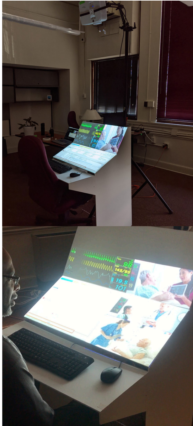
Fig. 2 Using projected images and videos to mockup a nurses station at full scale
