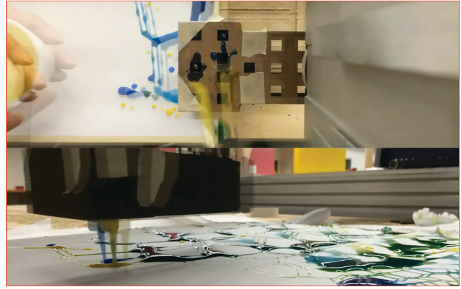
Figure 4. The Drip-jig with 2 color holder.
