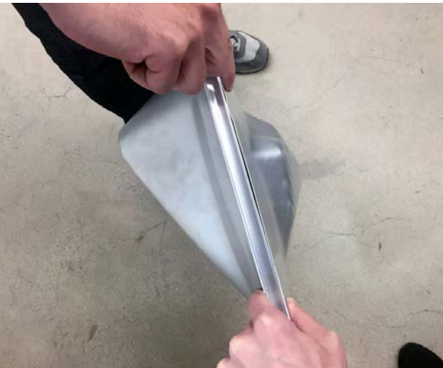
Fig. 29 U-shape channel between panels. It adds rigidity and absorbs deformations due to the stretch of the material.
