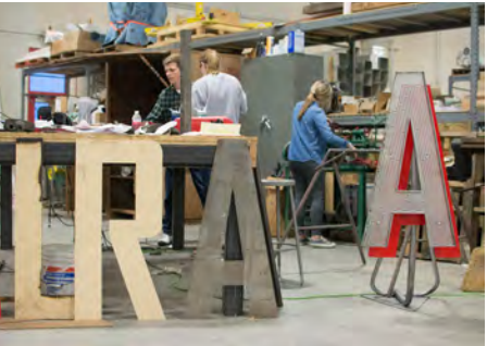
Fabrication of final signage system. Letters were plasma cut from solid and perforated metal sheets. CNC-cut MDF templates were produced to guide plasma cutting.
