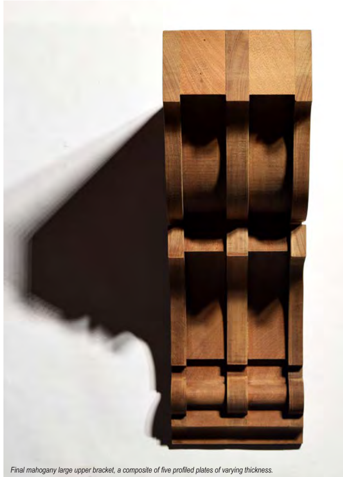
Final mahogany large upper bracket, a composite of five profiled plates of varying thickness.
