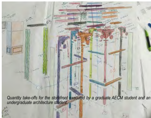
Exploded drawing differentiating parts according to material source and pre-fabrication processes generated in collaboration between undergraduate architecture students and graduate construction management students.
