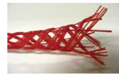
Epoxy-Cured shape detached from machine: 3 sets of 3 threads each constitute a total 20 threads wrapped to form the skeleton.
