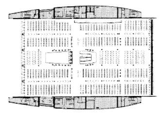
Fig. 2. The Phoenix Central Library: 5th floor plan with flanking saddlebags on the east and west sides of the main reading room.
