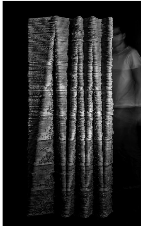
Figure 2. Smart Poche Wall variations (top left), Cluster section (bottom left), Smart Poche Wall full-scale 3D printed concrete prototype (right). Leslie Lok.
