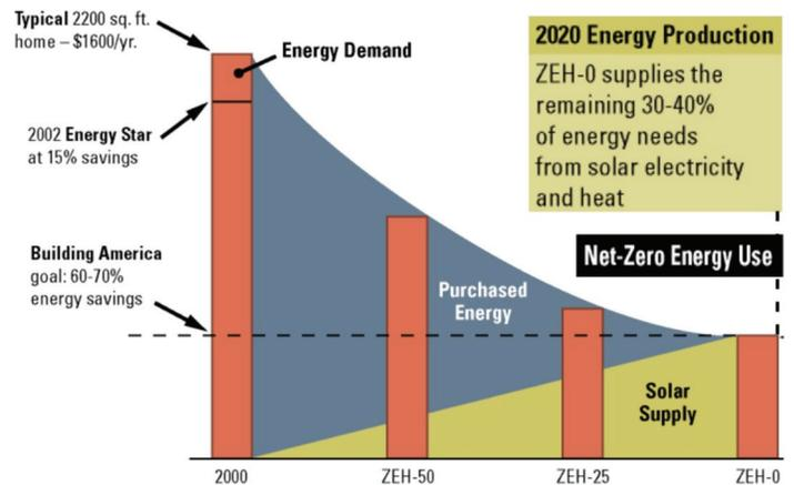
Figure 4. Progression to Full ZEH: Requirements in Building Codes and Policies for New Buildings. Source: Laustsen, IEA-2008. [http://www.iea.org/g8/2008/Building\\_Codes.pdf](http://www.iea.org/g8/2008/Building_Codes.pdf) , accessed on 3/28/2012
