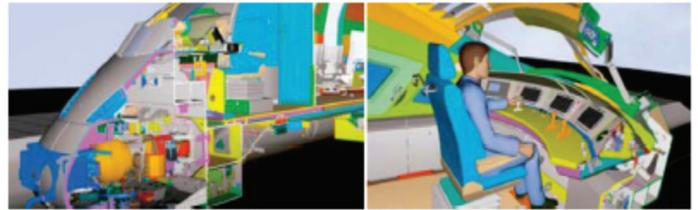
Figure 9. ICE-High Speed train nose section (left), ergonomics study of the driver's cab (right). Source: Siemens, pictures of the future, fall 2008.
