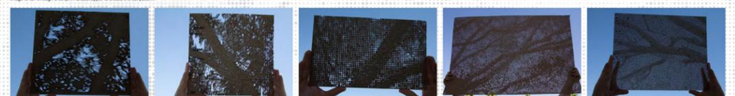
Students experimented with different perforation shapes and densities before deciding upon the final pattern. Using chipboard samples, the pieces were cut using a 100 watt laser which was the most appropriate laser method as the final panel panels were cut with a high power laser.
