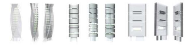
FIG. 5 (left to right) Three tower typologies proposed within the Ravenous Urbanism framework. Within tower mass, a variety of unit sizes and tenure types are accommodated including vertical greenhouse spaces and terrarium types with photovoltaic skins, and turbine types that generate energy to drive public amenities in vertical configurations, or at the space of the socle landscape below.
