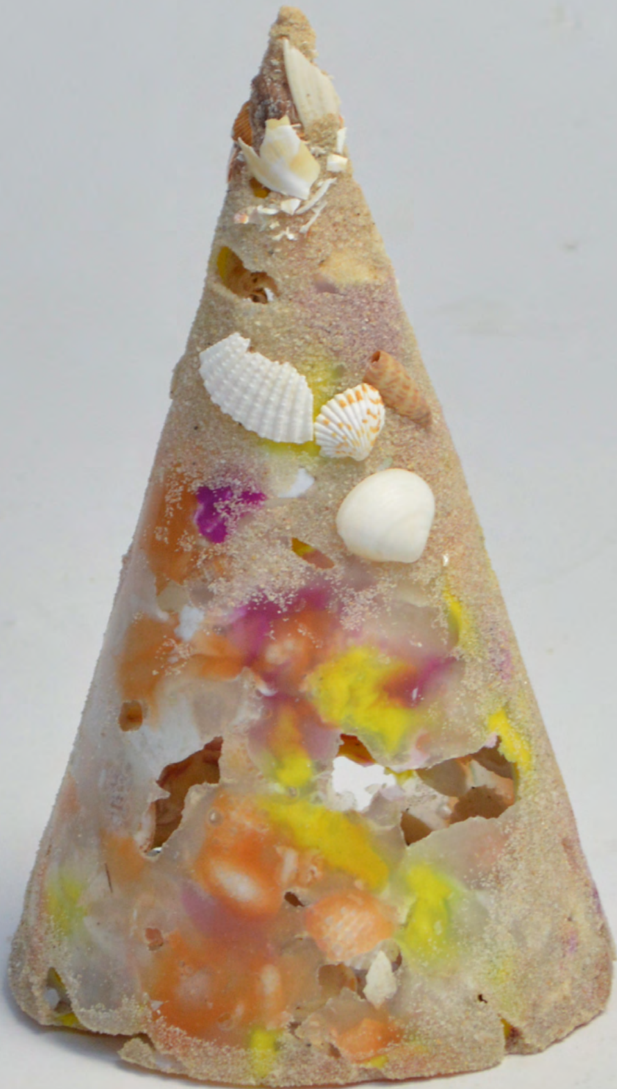
Scale prototype testing sand and plastic ratios
