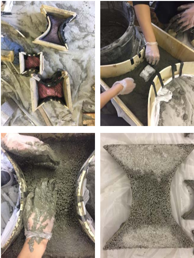
Pic - steps of fabrication process to create two layered system of bent forms.
