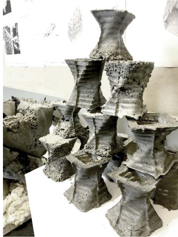
Pic - stacked forms of hybridized concrete forms (mixture of high strength, porous and/or lightweight concrete mixes)
