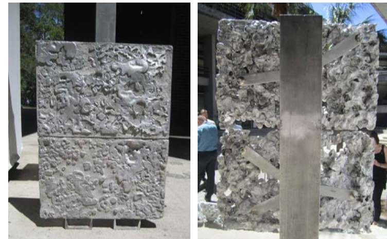
Ice casting aluminum + Aluminum cast into concrete
