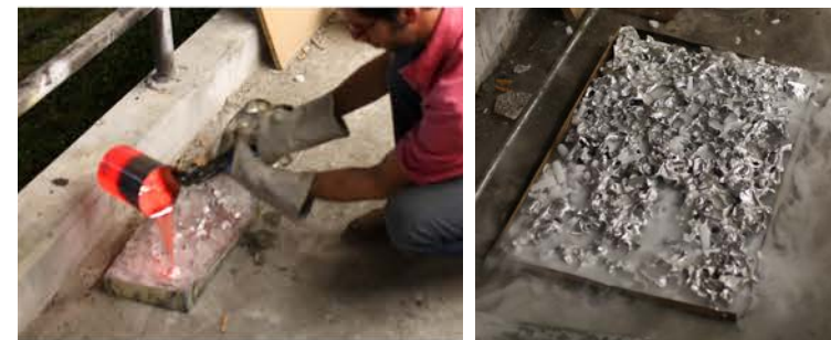
Ice casting aluminum + Aluminum cast into concrete
