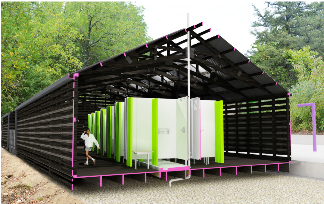
PLAN AND SECTION PERSPECTIVE The program called for 8 showers (1 ADA accessible), 4 changing stalls (1 ADA accessible) and storage cubbies for 50 girls. A 40' long continuous shower pan allows a flexible arrangement of showers.
