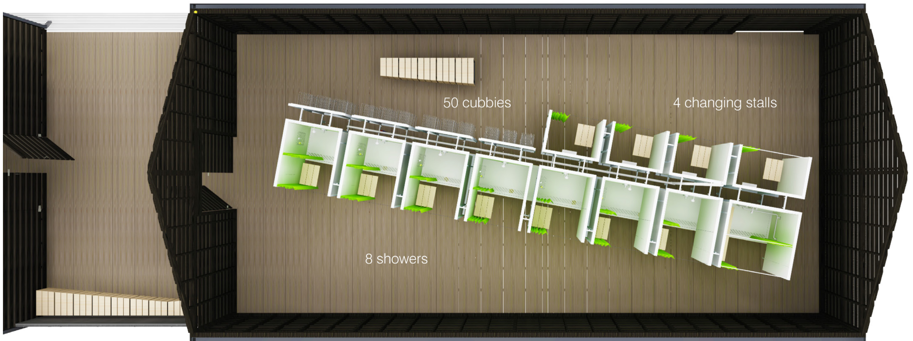
PLAN AND SECTION PERSPECTIVE The program called for 8 showers (1 ADA accessible), 4 changing stalls (1 ADA accessible) and storage cubbies for 50 girls. A 40' long continuous shower pan allows a flexible arrangement of showers.
