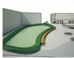
Water is now pumped into Marsh 1, which contains both aerobic and anaerobic bacterial environments. This is comprised of plants with a high tolerance to and capacity for contaminants (aerobic) and bacteria colonies known as bio films that attach to the root structure of the plants and aid in waste removal (anaerobic). A recirculating pump under the gravel moves water from bottom to top to increase dissolved oxygen, and stimulate nitrification and oxidation.
