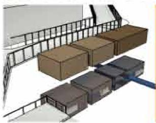
Solid materials start to settle while naturally present anaerobic bacteria begin to break down carbon and nitrogen-containing solids and liquids. This process converts organic nitrogen into ammonia. The remaining undigested solids are deposited in the bottom of the tank as sludge and the liquids are poured off. After this process is repeated in tank two it is passed through a bio-filter before entering tank three. The water is now ready for the Marsh Machine.
