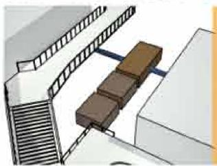
Waste water from the campus is piped into the first of three underground precast concrete holding tanks.
