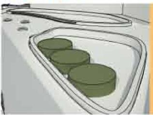
These three white tanks hold 550 gallons of water each and are highly aerobic environments, promoting bacterial floc formation and nitrification. The majority of the carbon is converted into bacterial biomass and the majority of the ammonia is converted to nitrate, some of which is consumed by the plants and algae.
