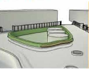
The same reactions occur as in Marsh 1, but this marsh is more anaerobic due to lack of recirculating pumps. The higher water level does not stimulate deep root growth, which would add oxygen to the marsh.
