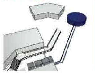
After the nearly potable water has passed through Marsh 2 it is passed through a final carbon particulate and UV light filter before it is deposited in the final holding tank where it is ready to be redistributed to the campus to be used for toilet flushing in all restrooms.
